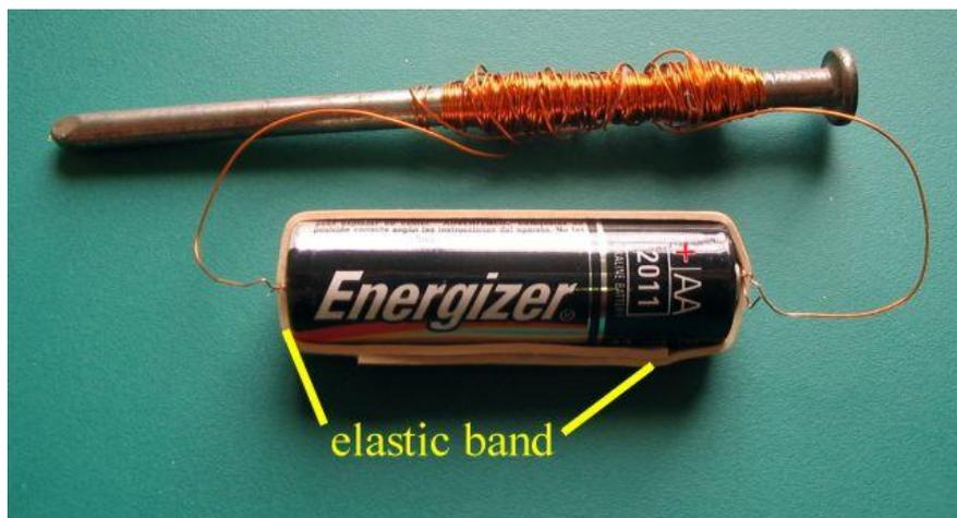
The elastic band holds each end of the wire against the battery terminals.
